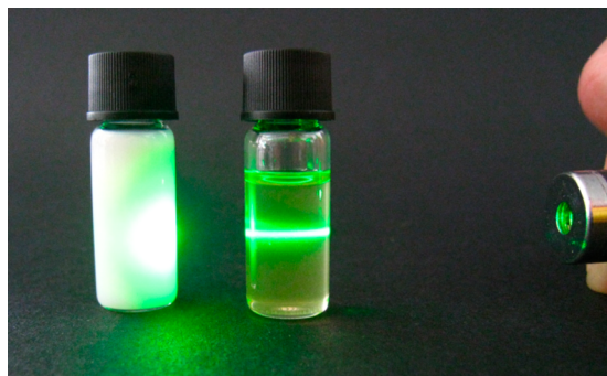
Figure 2. Dispersion of PS nanoparticles with surface-attached chromophore BTBD in THF (left) and the same particles as clear dispersion in isorefractive 2-ethylnaphthalene (right) illustrated with a commercial green laser pointer.
